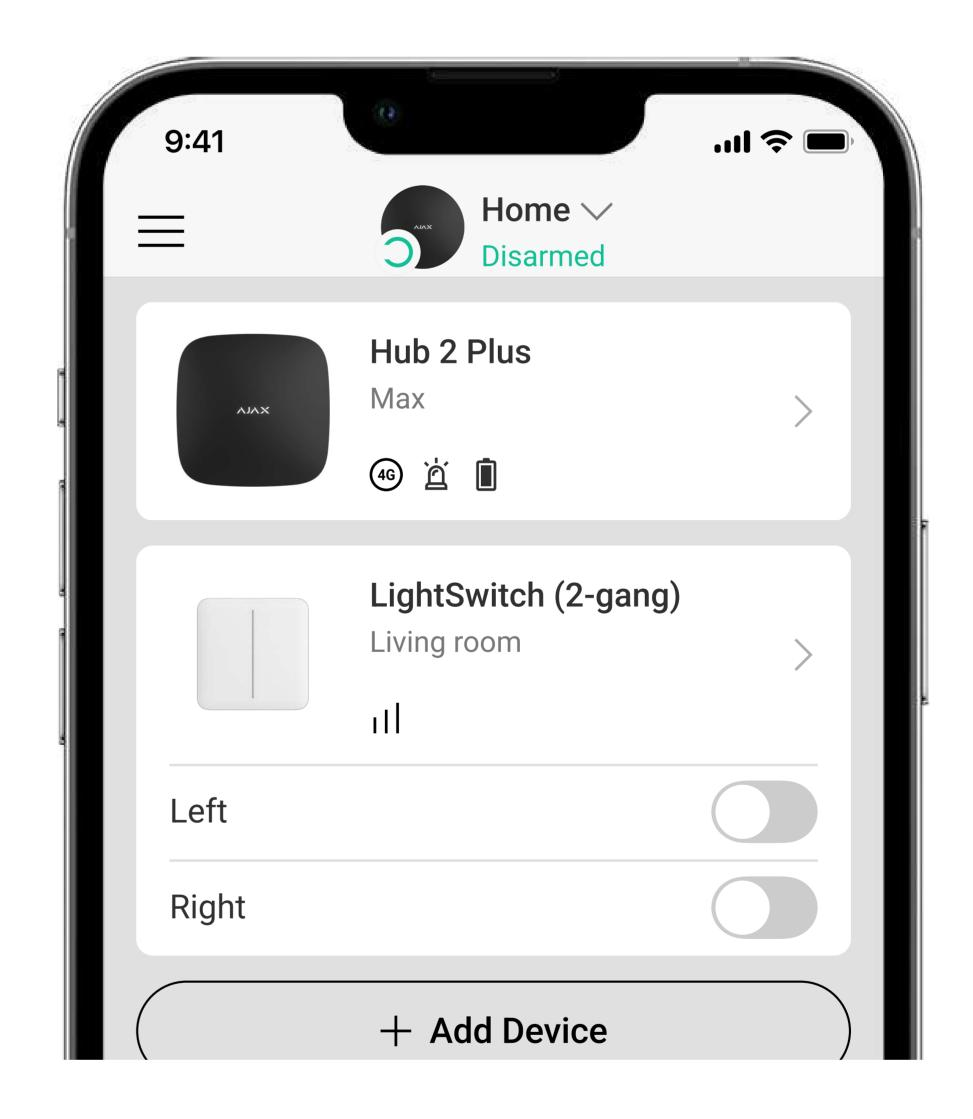
Installers can also configure the actions of automation devices by pressing LightSwitch. For example, in case of a blackout in the room, Relay activates the closing of the roller shutters.
